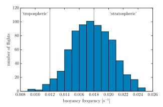
FIG. 1. Histogram of flight-average buoyancy frequency for MOZAIC flights with no selection for altitude as in Callies et al. (2014). The vertical lines indicate the thresholds for buoyancy frequency used in this paper for the classification of flight segments into tropospheric and stratospheric.
